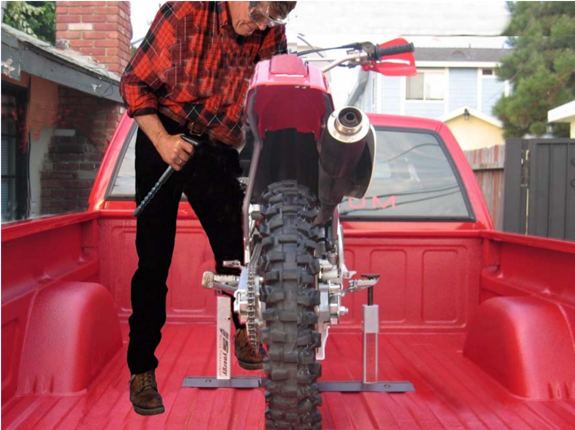
Figure 10: Motorcycle Positioned and P-LOK™ Rod Inserted
