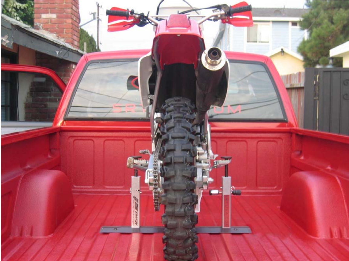
Figure 11: Motorcycle Secured by P-LOK™ System Ready for Transport
